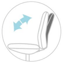
Back Angle with 4 Position Tilt Lock
